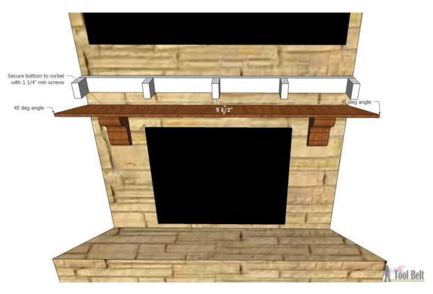
Cut the front board (casing) to fit snug along the bottom board and with a 45 against the walls. Nail the front to the bottom near the bottom edge with  $1 \frac{1}{4}$ " brad nails. Limit the number of nail holes, since they'll show (probably about 4-5). Nail the front to the mantel support 4" 2x4's near the top 2" or so. The crown will cover these holes.
