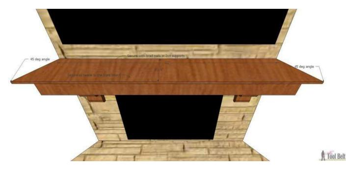
Cut the crown molding to fit under the top. Nail the crown in place, with as minimum nails as possible.
