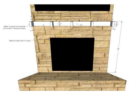
Cut a piece of 2x4 to 62" and cut 5 pieces that are 5" long. Spread the 4" pieces evenly along the 2x4, and secure from the back of the 2x4 with 3" screws (make sure they are countersunk or sucked into the wood). Mark the studs in the fireplace wall, level and attach the mantel support into the studs with 4" screws. (I attached it at 45" from the step)
